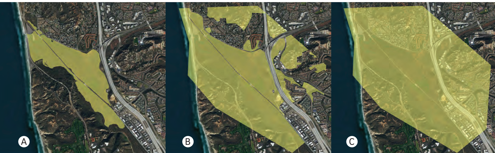
Figure 12. Map visualization of the footprints used in the analyses for each wetland migration scenario: (A) no wetland migration, (B) wetland migration avoiding developed areas and (C) wetland migration including developed areas in Los Peñasquitos.
