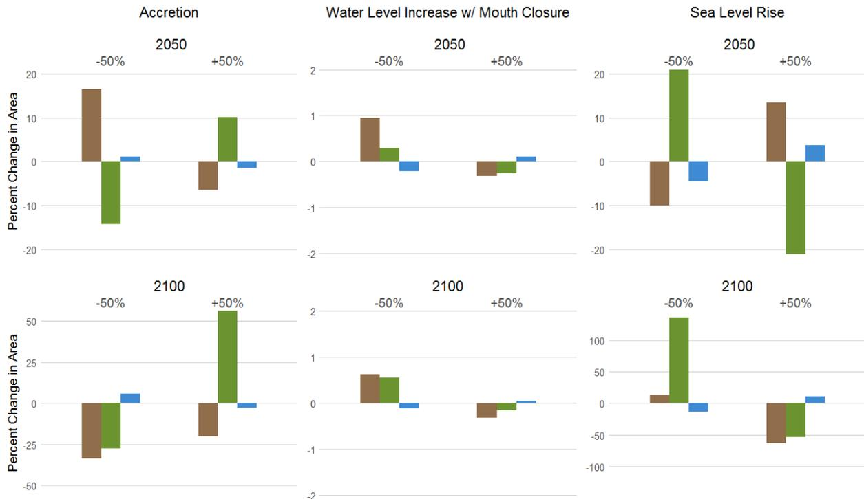
**Figure 16. Percent change in habitat area caused by sensitivity to model inputs. Changes to subtidal (blue), unvegetated mudflat (brown), and vegetated marsh (green) habitats when model inputs (Accretion, Mouth Dynamics, SLR) are increased (+50%) or decreased (-50%). Note varying y-axis scales in plot panels.**
