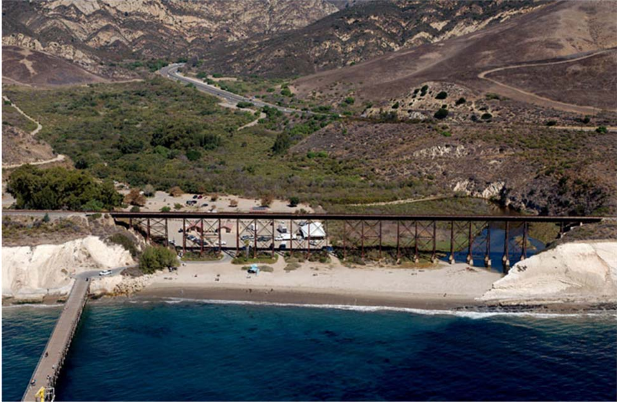
Figure 4. Past alterations to small creeks illustrated by Canada de la Gaviota Creek - railroad crossing, jetty, inlet armoring and parking lot fill (Photo: California Coastal Records Project, 2013).
