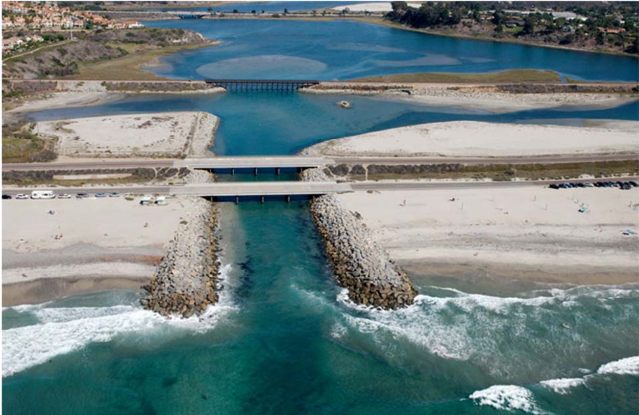
Figure 6. Alterations at Batiquitos Lagoon (Photo: California Coastal Records Project, 2013). Roads, railroad, and jetties have significantly changed the natural cycles at this wetland. The jetties were built as part of a previous project to restore wetland habitat at the lagoon.
