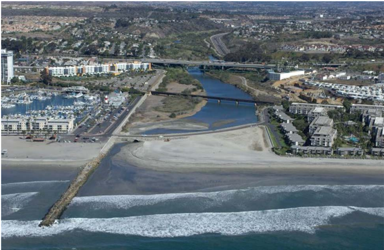
Figure 7. Intermediate estuary - San Luis Rey River with a tidal inlet highly controlled by the Pacific Street bridge. (Photo: California Coastal Records Project, 2013)
