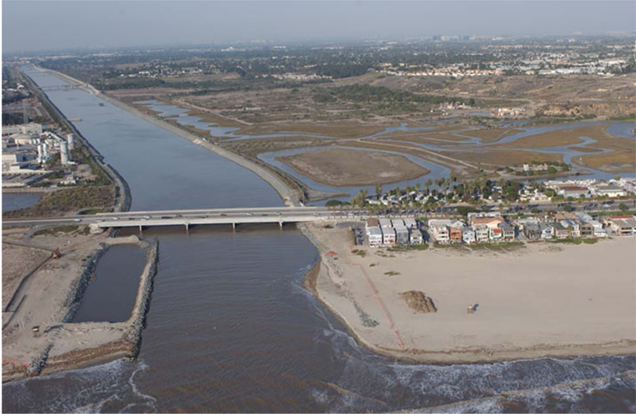
Figure 8. Past alterations to large river valley estuaries - Santa Ana River rerouted and the Santa Ana wetlands fragmented by the construction of the flood control channel. (Photo: California Coastal Records Project, 2004)
